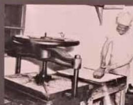
工人將玉扣紙鋪在鉛字盤上，壓印成紙版。 "Yukou" paper is placed on the moveable lead type plates and the characters are embossed on the paper.
